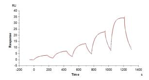
Biotinylated Human FGF10, No tag immobilized on CM5 Chip can bind Human FGFR2 alpha IIIb, His tag with an affinity constant of 147.70 nM as determined in SPR assay (Biacore T200) (QC Test).
